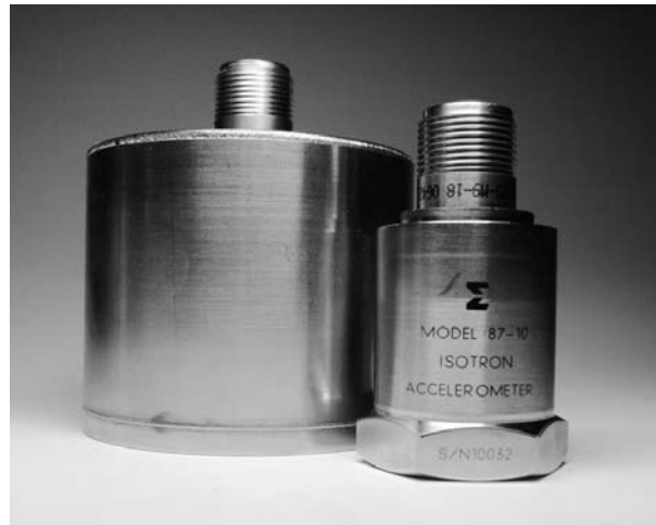
Figure 2 Showing the Endeveco models 86 and 87 low-noise accelerometers. Note the large size of the model 86, which is the ultra low-noise unit.
