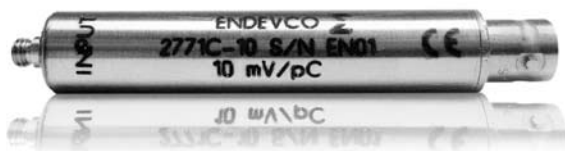
Figure 3 Endevco 2771C low-noise charge converter with 10-32 Accelerometer connector and BNC for the conventional two wire IEPE output/power
