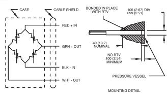
STANDARD TOLERANCE INCHES (MILLIMETERS) .XX = +/- .03 (.X = +/- .8) .XXX = +/- .010 (.XX = +/- .25)
