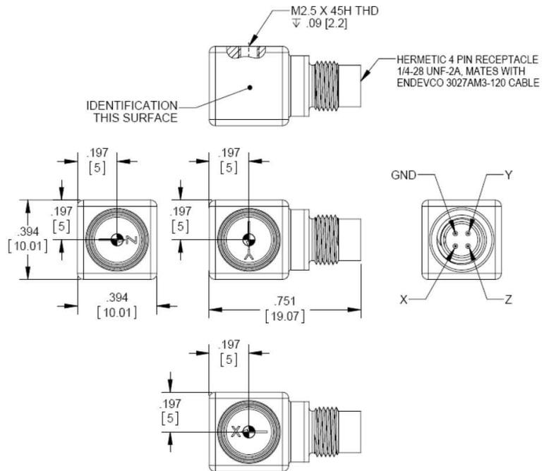
⊙ INDICATES LOCATION OF SEISMIC MASS
