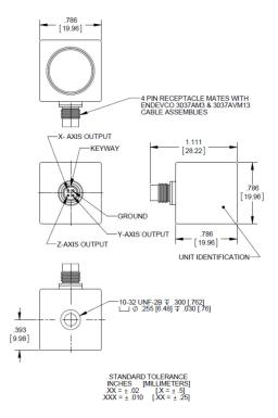
Model 45A is a cost effective general purpose triaxial lsotron accelerometer designed for use in a variety of applications. 45A is a 20 mm cube shaped lsotron accelerometer, featuring a single threaded 1/4-28 4 pin connector.
