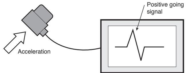
Figure 4: Output polarity
