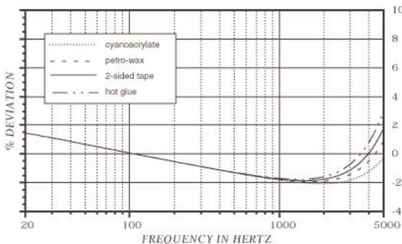
Figure 1 Frequency response curves with various adhesives
