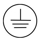
Protective conductor terminal. For protection against electrical shock in case of a fault. Used with field wiring terminals to indicate the terminal which must be connected to ground before operating the equipment.
