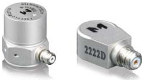
Figure 5 Shown on the left is a popular side connector accelerometer that weighs 7.8 grams and is used on heavy test articles. The unit on the right is a miniature accelerometer that weighs 0.5 grams that can be mounted on lightweight structures and PC boards.
