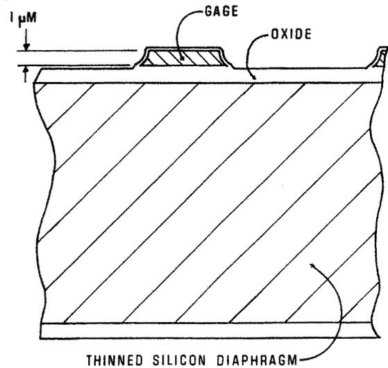
Figure 3 Oxide-bonded gage
