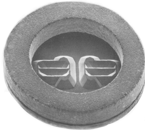
Figure 3 — Photograph of diaphragm, glass-bonded to heavy silicon ring, 0.1 in (2.5 mm) O.D. by 0.02 in (0.5 mm) thick.
