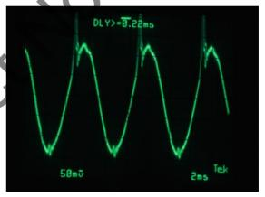
Figure 7A: Acceptable sine wave from reference mate.
