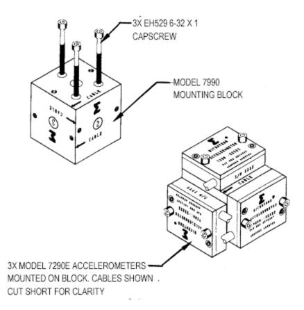
FIGURE 2- Installation of (3) Model 7290E Microtron Accelerometers onto Model 7990 Triaxial Block
