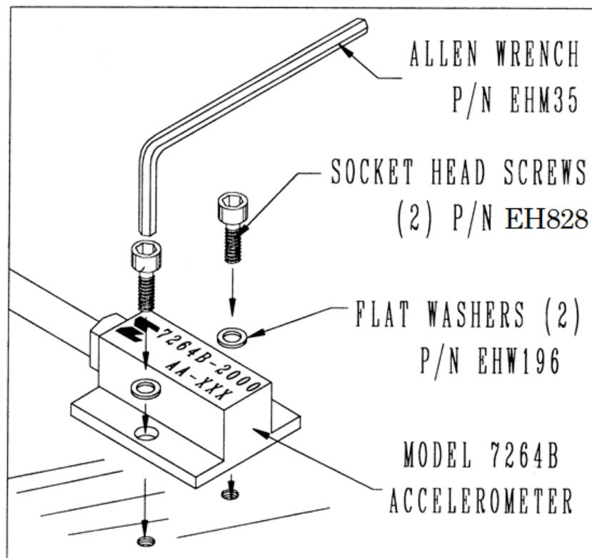
**FIGURE 1 - Installation of Model 7264B Accelerometer**
