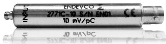
**Figure 3** Endevco 2771C low-noise charge converter with 10-32 accelerometer connector and BNC for the conventional two wire IEPE output/power
