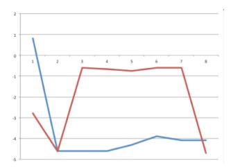
*Chart 1: ZMO shift in mV vs. time in days. Red trace is concentrated antifreeze and the blue is tap water. Some of the initial shift is attributed to temperature change.*
