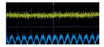
*Figure 3:* Yellow trace is the transducers noise level before ingression. The blue trace shows the noise level after water ingression.
