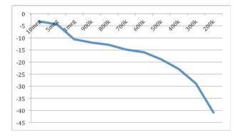
Chart 2: Effect of loading the output of a 8510B pressure transducer. At 10 meg  $\Omega$  the ZMO has returned to its pre-resistive loaded value.
