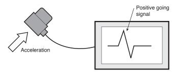
Figure 4: Output polarity
