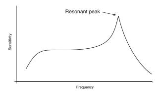
Figure 3: Mounted resonant frequency
