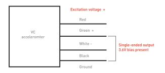
Showing proper connections for a single-ended Figure 4 output. An amplifier with a single-ended input is connected to the green and black leads.
