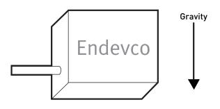
Figure 2 Showing a typical Endevco VC accelerometer on its side. This is the "zero g" position.
