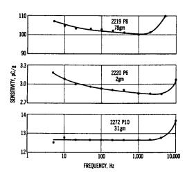
Figure 3-6 Charge frequency response characteristics of piezoelectric accelerometers representing various accelerometer designs and crystal materials.
