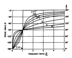
Figure 3-3 Phase angle response of seismic accelerometer indicates the relative displacement,  $\delta$ , to the applied acceleration, u.
