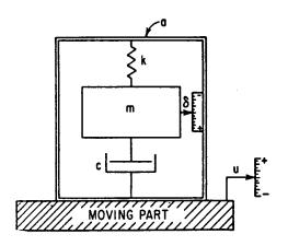
Figure 3-1 Single-degree-of-freedom seismic accelerometer consisting of a mass element M supported by spring K with damping C. The case of the accelerometer is attached to the moving part whose motion is to be measured.
