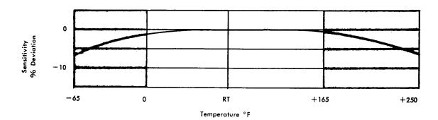
Figure 3-14 Typical sensitivity changes of a piezoresistive accelerometer as a function of temperature.
