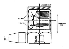
Figure 3-12 Sketch of a piezoresistive strain gage accelerometer.
