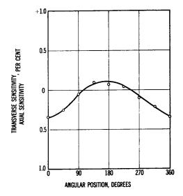
Figure 3-11 Variation in transverse sensitivity as a piezoelectric accelerometer is rotated about its sensitive axis.
