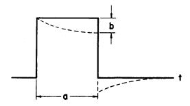
Figure 2-15 Theoretical responses from accelerometers exposed to long-duration square wave shock motions.
