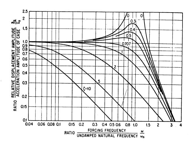
Figure 3-2 Frequency response of an accelerometer subjected to sinusoidal motion.
