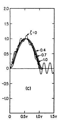
Figure 3-16 Response of accelerometers to short duration half-sine shock pulses.
