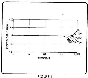
Comparison Calibrations performed to determine the relative motion present in the 2270 accelerometer standard as a function of test accelerometer mass.
