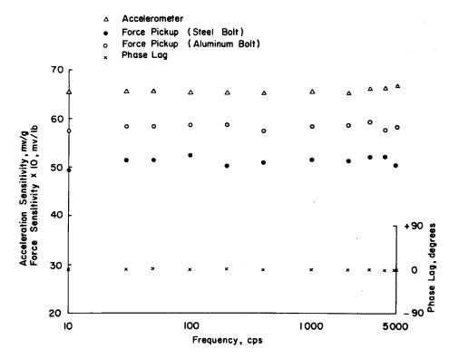
Figure 3. Calibration results on an impedance head. The force pickup and accelerometer were calibrated by comparison with a standard accelerometer. The phase angle measurements were made with a dual-beam oscilloscope.
