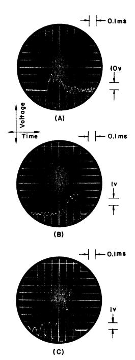
Figure 6. Resonance response of an impedance head. (A) Resonance frequency of the accelerometer part of the impedance head is 28,000 cps. (B) and (C) Force response with the impedance head mounted in two structures resonate at 20,400 cps and 10,300 cps, respectively.
